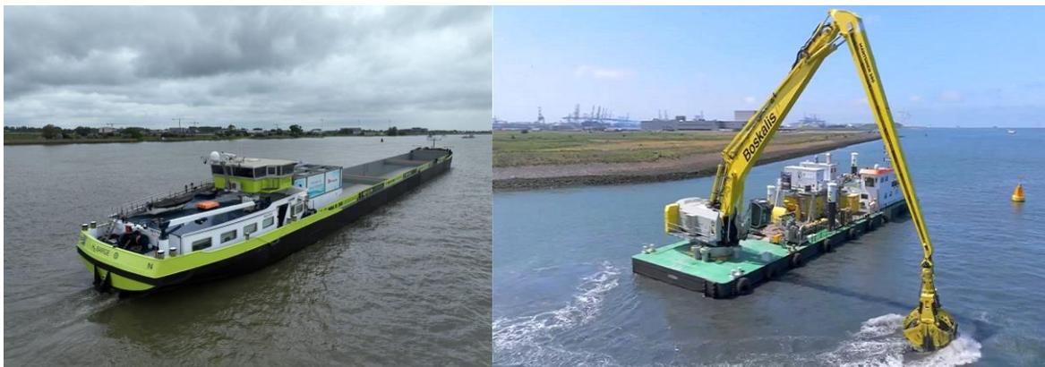
Two operational vessels equipped with hydrogen fuel cells: H2 Barge 1 (left) and Medusa 2 (right)<sup>18</sup>.
