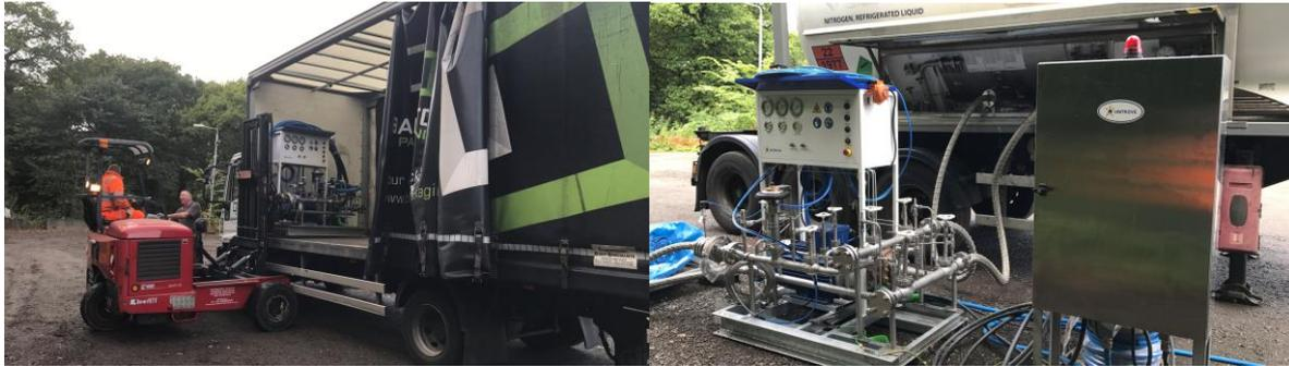
*Unitrove's zero emission multi-fuel system (ZEMFS) condenses bunkering infrastructure onto the back of a truck to enable flexible and low-risk refuelling<sup>15</sup>.*
