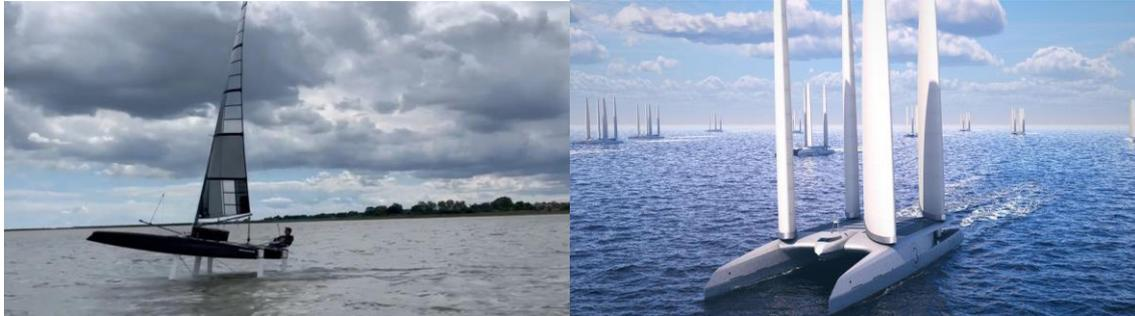
*Drift Energy's demonstrated mobile green hydrogen production vessel prototype (left) and 2 MW full scale design (right)<sup>14</sup>.*
