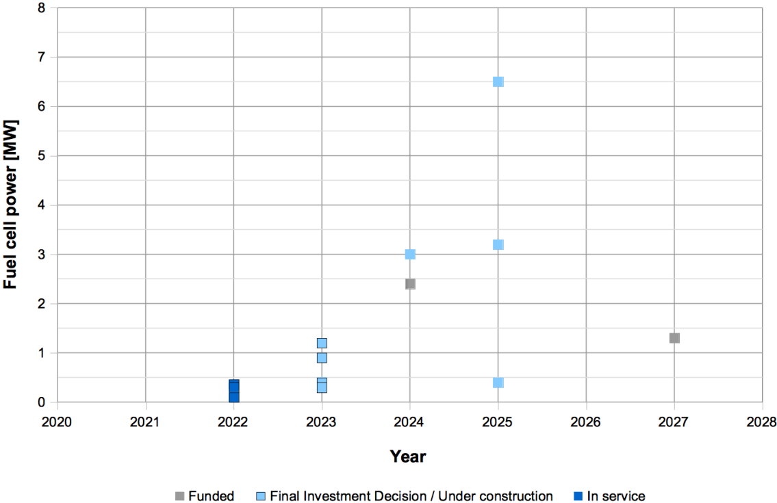
Figure 3: Installed fuel cell system nominal power outputs for existing and expected vessels.
