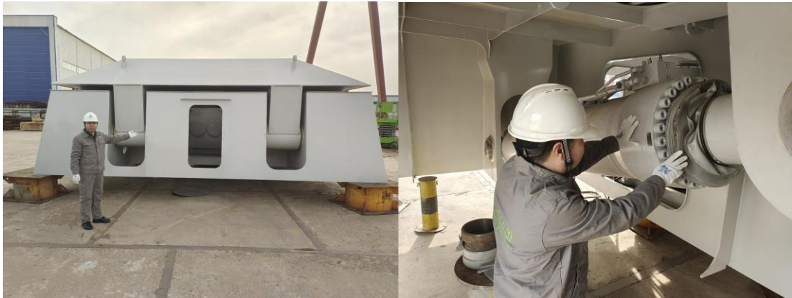
Figure 26: Example of folding rotor sail foundation including the tilting system cylinder. Image: Dealfeng New Energy Technology Ltd.).
