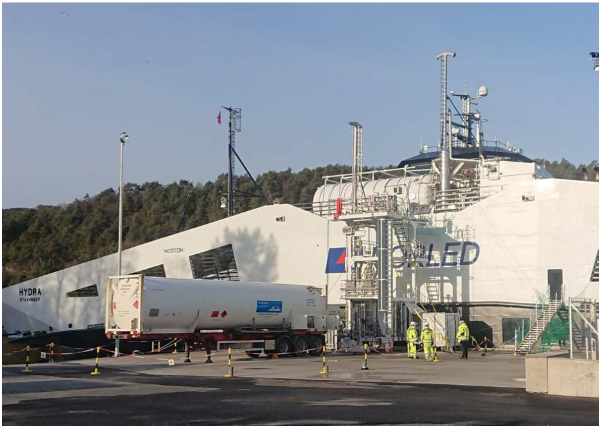
Norled mobile bunkering tower delivering liquid hydrogen to Hydra RoPax ferry using trailer.
