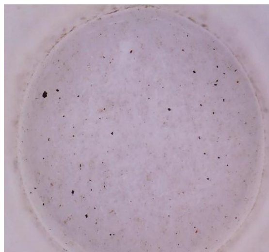
Fig. 4. 1000 particles of black carbon particles per litre of water; collected in the equatorial Atlantic Ocean. Ref 18
