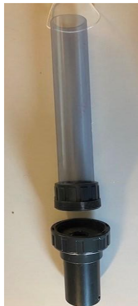
Fig. 7. GOES plankton sampler
