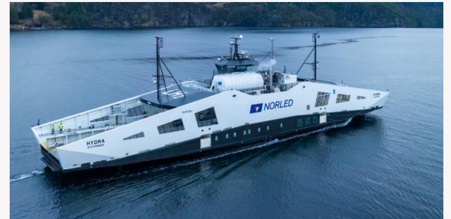
M/F Hydra, world's first ship sailing with LH 2 as fuel. Ship and technology certified by DNV (class) and NMA (Flag). Picture: Norled
