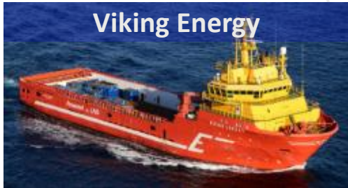
PSV with battery power
