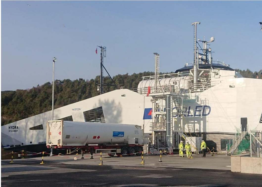
Figure 6: Mobile liquid hydrogen bunkering tower designed and owned by Norled attached to a tube trailer, bunkering the Hydra passenger ferry. (Credit: Norled)
