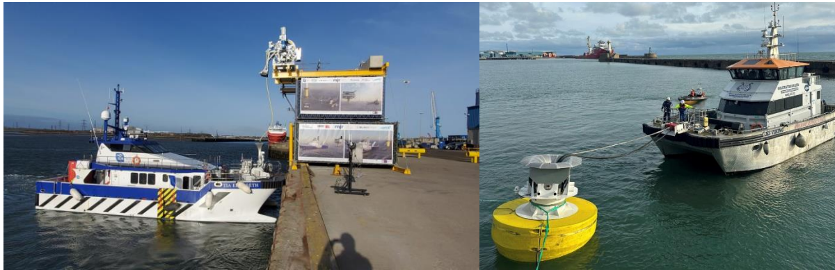
Figure 3: Harbour trials of offshore charging systems. Left: 1.5 MW charging point to be fixed on an offshore structure (image: MJR Power & Automation). Right: floating buoy charging point (image: Jebb Smith Ltd)
