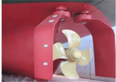
GATE RUDDER SYSTEM (GRS)
