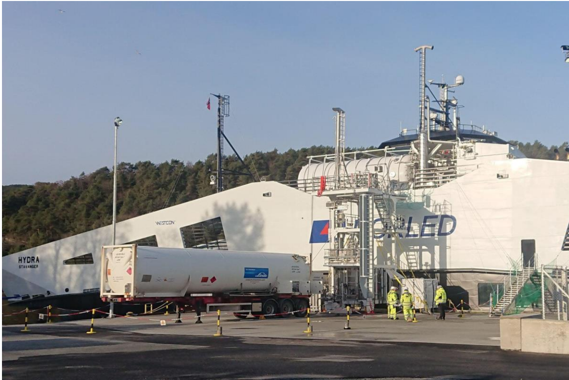
Figure 20: Mobile liquid hydrogen bunkering tower designed and owned by Norled attached to a tube trailer, bunkering the Hydra passenger ferry. Image: Norled AS.
