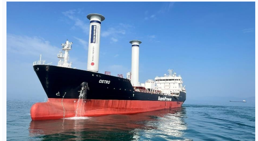
Ostro – Rotor Sail Fitted Intermediate Chemical Tanker
