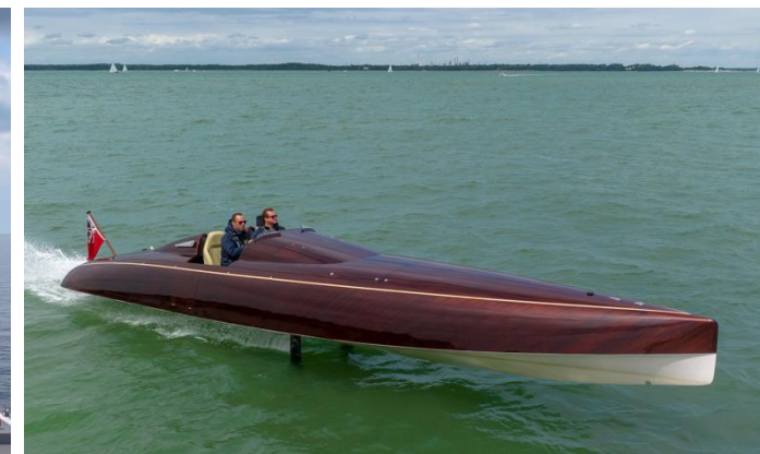
BARTech Spirit F35: Electric foiling launch
